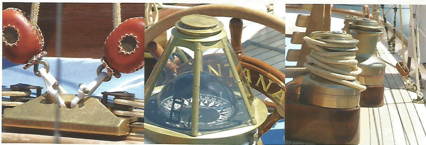
Above left to right: leather-clad blocks by Ording; original binnacle; new bronze winches by Harken
